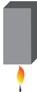
Vertical Burn Self Extinguishing UL 94 V-0 (Best) UL 94 V-1 (Good) UL 94 v-2 (Drips)
