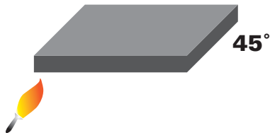
Horizontal Burn Slow Burn Rating Takes more than 3 min. to burn 4 inches
